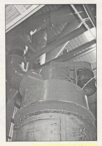
This roller mill, fitted with a conversion classifier, gives workers better control over the top size cut of fine particles. It also lifts the fine particles out of the grinding zone more quickly, thus increasing efficiency and throughput.
