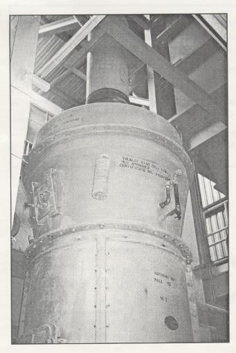
This roller mill is still using its original classifier. Without varible-speed motors on the fan or rotor, workers use dampers to control air volume and thus control particle size.
