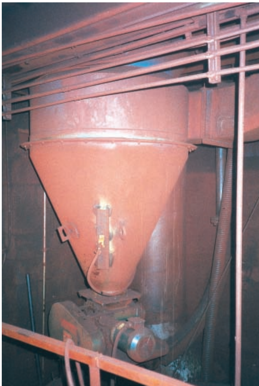
The MS-20 Micro-Sizer air classifier (here covered with red iron oxide dust) can handle up to 20 t/h of material, as well as produce cuts as fine as 100 percent less than 10 microns on most materials.
